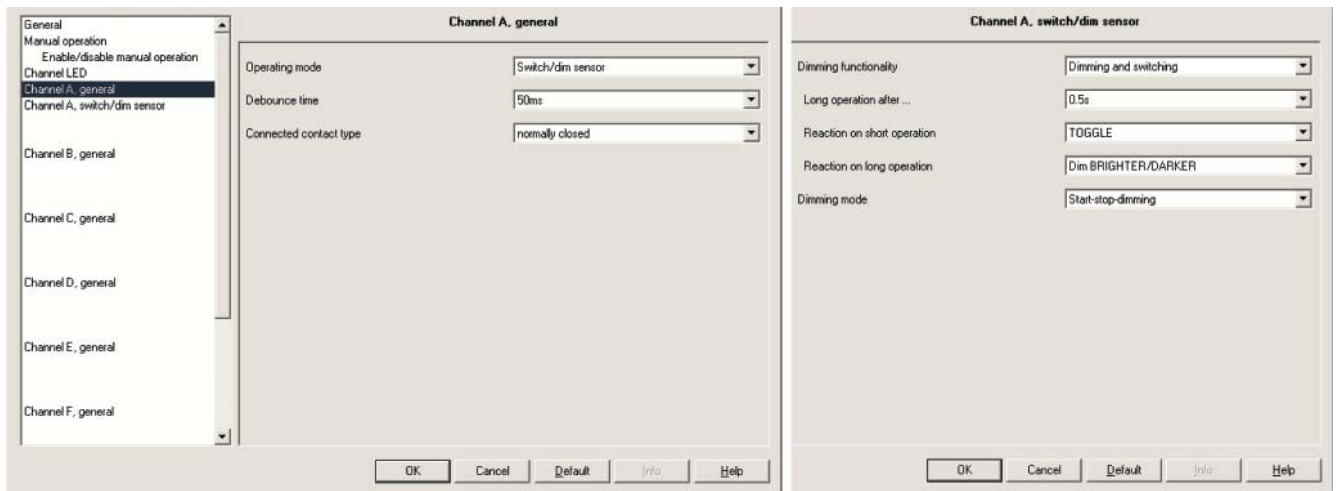
Fig. 86: 1 button operation of lighting (dim lighting)
